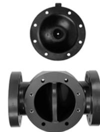
If 60PSI or more pressure is used with the 4" (d110) PTFE valve additional torque should be applied to all 8 bolts. The appropriate valve is 33% greater or 354 inch lbs (40 Nm). No more than 354 inch lbs should be applied to the bolts. Please contact us with any further questions or comments.
